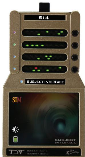
**Overview.** TDT's Subject Interface [SI] is an exciting new hybrid device capable of both electrical stimulation and biological signal recording. The SI can be tailored to meet the unique needs of your research by combining different banks of electrical stimulation, analog recording and digital headstage inputs. The SI comes in different "sizes" that vary by the total number of banks. Choose between our 2, 4, 6 and 8 bank SI models, depending on the capacity your research requires.
