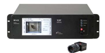
**Software Control.** Software control is implemented with circuit files developed using TDT's RP Visual Design Studio (RPvdsEx). A single RPvdsEx macro is provided to configure the RZ to send trigger information to the RV2 and receive frame and positional information.
