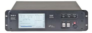
Software Control. Software control is implemented with circuit files developed using TDT's RP Visual Design Studio (RPvdsEx). Circuits are loaded to an RZ processor through TDT run-time applications, such as OpenEx or custom applications via ActiveX controls.
