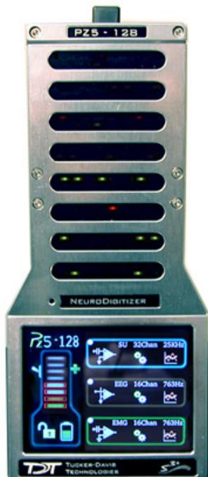
**Overview.** The PZ5 is a multi-modal neurodigitizer suitable for recording a broad range of biological potentials. Its analog input boards combine the functionality of the PZ2 and PZ3 amplifiers in a single device that can be used for both high and low impedance input signals simultaneously. The PZ5 may also include digital input boards for inputting signals from an Intan RHD2000 amplifier board with up to 128 channels.
