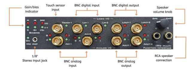
The iM5, iM7, iM8, iM9, iM14, and iM15 have specialized I/O functions, including advanced audio processing critical for auditory behavioral experiments.
