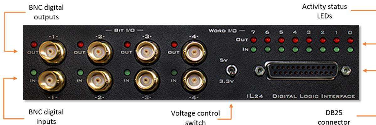
The iL24 module can communicate with external behavioral components using 24 bits of 5 V or 3.3 V TTL logic signals. There are 12 input bits and 12 output bits. Each direction has 4 addressable bits and 1 addressable byte.
