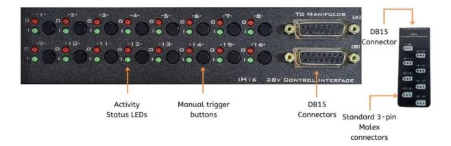
The iH16 and iH8 modules feature 16 or eight bidirectional interface ports to directly control high-voltage (e.g. 28 V signal) cage elements including Med Associates, Lafayette, and Coulbourn. The iH8 and iH16 modules connect to an iHm, iH8-RJ25PLA/B, or iH8-RJ25A/B manifold via a DB15 cable. The manifold can be placed closer to the behavioral apparatus.
