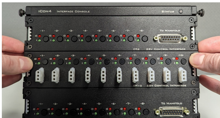
Example grip for removing the top module. Pull the module tabs on both sides while bracing against lower modules
