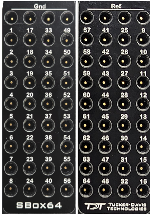
Front and back pinout of S-BOX64
