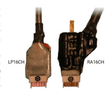
The LP16CH-ZNF uses non-ferrous materials, including a non-ferrous Omnetics connector with the same size and pinout as the RA16CH and LP16CH headstages. It can be used for recording single-unit electrophysiology during fMRI neuroimaging.
