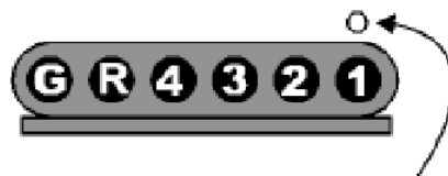
Channel 1 marked with a dot on probe head
