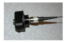
4. Disconnect the fiber from the joint.
