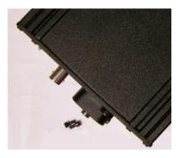
2. Use the hex driver to remove two screws securing the encoder clamping plates.
