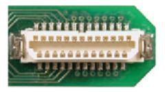
Two or four interface receptacles are positioned on the rotary interface module. The receptacles are labeled to correspond to the DB26 connectors on the face. The ACO32 uses 'A' and 'B' labels, the ACO64 uses 1 to 4 silver marks on the receptacles. TDT offers headstages and connectors with a mate for these receptacles.
