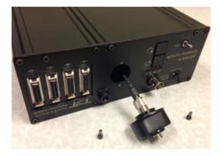
2. Use the hex driver to remove the two screws securing the encoder clamping plates.
