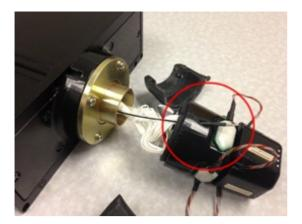
4. Secure the two encoder clamping shells back onto the ACO64 shaft by inserting and tightening the two screws.
