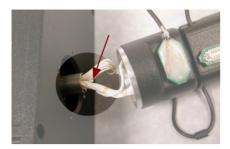
3. Using a pair of tweezers, carefully pull the end of the fiber and insert it into the hole next to the encoder.
