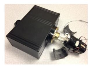
3. Carefully pull the FORJ away from the commutator face until the fiber is free.
