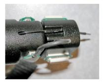
5. Leave enough slack in the section of fiber between the encoder and connector modules to match the loop of the other wires. A small lightweight tie can be loosely attached to hold the fiber adjacent to the wires.
