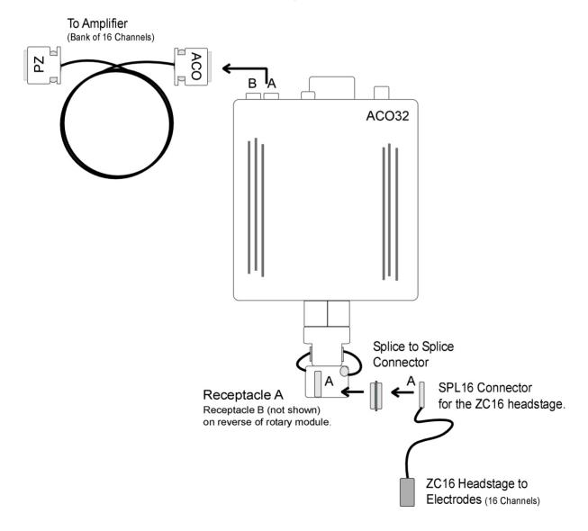
The diagram above shows the ACO32 connection for the A subset of channels:
