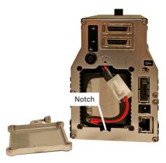
2. The connector between the batter pack and the device will be immediately visible. Press down on the tab to release the connection then gently pull the battery pack free from the device.
