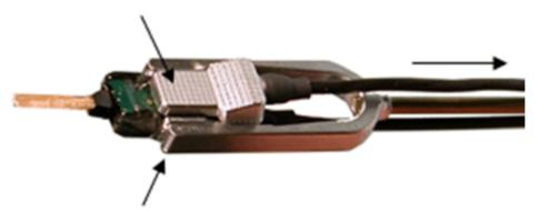
To remove, grip the top and bottom of the headstage and gently slide the holder away.
