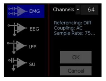
Select the Amp Type and set the number of channels in the logical amplifier (by banks of 64 channels for analog amplifiers).
