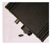
2. Use the hex driver to remove two screws securing the encoder clamping plates.
