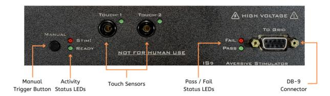
The iS9 generates small electrical currents for standard behavioral conditioning experiments, such as startle and Pavlovian fear response. Timing is precisely controlled for pairing the stim with other sensory cues or behavioral events. The iS9 is compatible with 3<sup>rd</sup> party behavioral boxes (Med Associates, Lafayette, and Harvard Apparatus).
