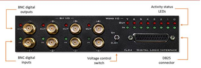
The iL24 module can communicate with external behavioral components using 24 bits of 5 V or 3.3 V TTL logic signals. There are 12 input bits and 12 output bits. Each direction has 4 addressable bits and 1 addressable byte.
