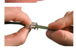
Align the **notch guide** of connector to the **black square guide** of the fully opened headstage then move headstage into position.
