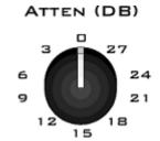
Manual attenuation is applied to both channels before the signals are output on any of the front panel connectors and is therefore applied in addition to any programmable attenuation.
