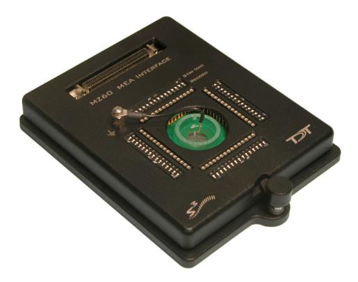
The MZ60 Microelectrode Array (MEA) Interface is used with our RZ2 BioAmp Processor and the PZ5 NeuroDigitizer (or SIM Subject Interface) as part of a complete solution for high spatio-temporal resolution tissue slice and cell culture recordings.
