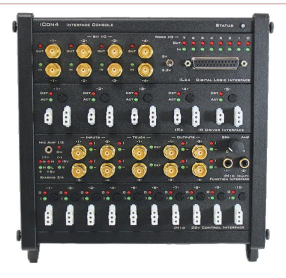
The iCon is a behavioral control interface designed to support easy or complex behavioral experiments. It has interchangeable analog and digital modules to fit the needs of any experimental paradigm. It can control most third-party behavioral chambers with TDT's Synapse software — resulting in high-bandwidth, precision control of behavioral hardware with real-time signal monitoring.
