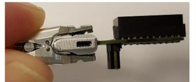
Align the **notch guide** of connector to the **black square guide** of the fully opened headstage then move headstage into position.
