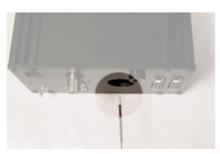
2. Slowly push fiber through hole until the end appears among the wires on the other side of the ACO32.
