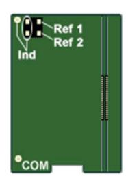
A four-pin header located on the backside of the adapter is provided for access to two probe reference pins. These pins are separate references and are connected internally to the adapter.
