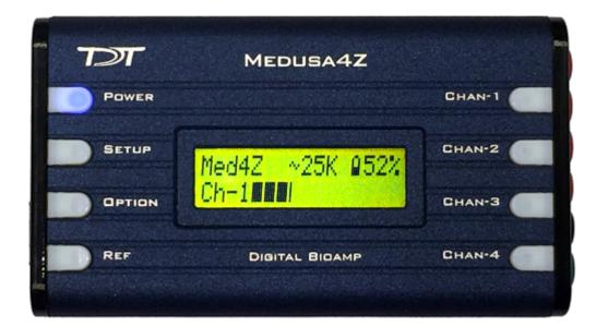
The LCD screen shows the current sampling rate, battery level, and signal level indication on the active channels.
