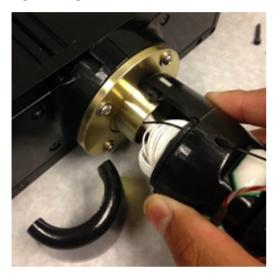
5. The plate should be just below the body of the ACO64 and the encoder body should sit snugly inside the lip of the clamping plates. Be careful not to pinch any wires or the fiber as the plates are tightened together.
