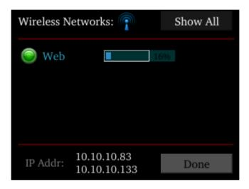
The Wireless Networks screen is displayed by touching WiFi on the System Setup screen. Available networks that have been used or previously configured are displayed in the main area of the screen. Selecting a network from the list displays network information and enables the user to connect to the network, forget the network, or cancel configuration of the network.
