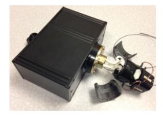
3. Carefully pull the FORJ away from the commutator face until the fiber is free.
