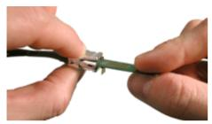
Align the **notch guide** of connector to the **black square guide** of the fully opened headstage then move headstage into position.
