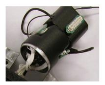
6. Connect the FC/PC connector end of the fiber to (the smaller section of) the fiber optic rotary joint.
