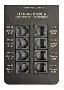
The iH8-RJ25PLA/B manifolds feature 8 telephone-style 6-pin RJ25 ports to provide direct control of high-voltage (e.g. 28V signal) cage elements from Panlab.
