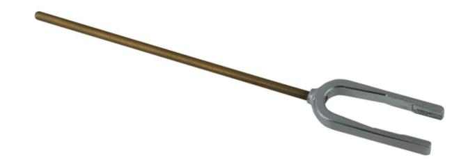
The ZIF-Clip® headstage holders securely hold your analog or digital ZIF-Clip® headstages during electrode insertion and can be used with most micromanipulators. The headstage holders, including the stabilizing rod, are approximately 4.5" in length. The stabilizing rod is 3" in length and has a 3/32" diameter. An aluminum lock pin ensures the ZIF-Clip® does not open during insertion.
