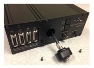
2. Use the hex driver to remove the two screws securing the encoder clamping plates.
