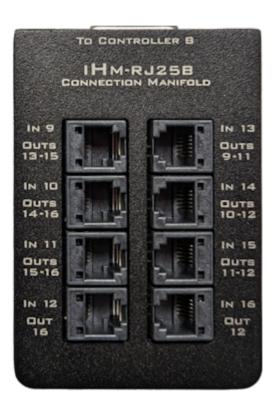
The iH8-RJ25A/B manifolds feature 8 telephone-style 6-pin RJ25 ports to provide direct control of high-voltage (e.g. 28V signal) cage elements from Coulbourn.
