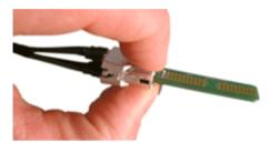
Press the **front** of the headstage together as shown to lock the connector in place. You should hear an audible click when the locking mechanism is engaged.
