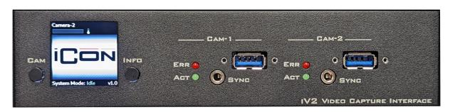
The iV1/iV2 iCon modules connect to USB3 cameras to record video frames synchronized with all behavioral, electrophysiology, fiber photometry, and other research data. Record video from up to two cameras simultaneously per iV2 module or one camera per iV1 module. The iV2 also features real-time subject tracking.
