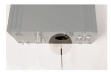
2. Slowly push fiber through hole until the end appears among the wires on the other side of the ACO32.
