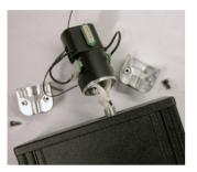
3. Carefully pull the FORJ away from the commutator face until the fiber is free.
