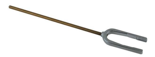
The ZIF-Clip® headstage holders securely hold your analog or digital ZIF-Clip® headstages during electrode insertion and can be used with most micromanipulators. The headstage holders, including the stabilizing rod, are approximately 4.5" in length. The stabilizing rod is 3" in length and has a 3/32" diameter. An aluminum lock pin ensures the ZIF-Clip® does not open during insertion.
