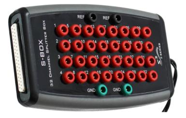
The S-BOX\_PZ5 is a 32-channel passive signal splitter for use with the PZ5 Amplifier or PZA (Subject Interface) Amplifier. The splitter provides a simple and effective means of routing low impedance biological signals to both a TDT acquisition system and a parallel recording system.
