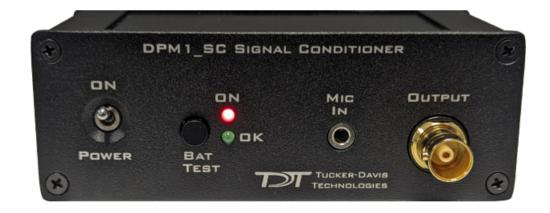
The DPM1\_SC is powered by two 9V batteries. Alkaline batteries are recommended. The "Bat Test" button on the front of the SPM1\_SC checks the battery level and lights the green "OK" LED when it is acceptable.
