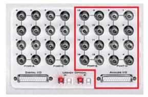
The RZ2 also includes onboard D/A for stimulus generation and experiment control, and A/D for input of signals from a variety of other analog sources.
