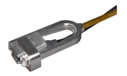
The U-shaped lock pin secures the connection and prevents the ZIF-Clip® from opening and releasing the probe.
