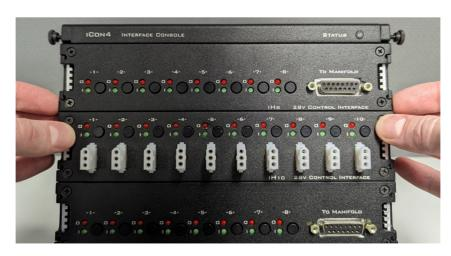
Example grip for removing the top module. Pull the module tabs on both sides while bracing against lower modules
