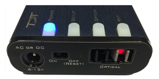
Use the provided fiber optic pair (black cable, white connectors) to connect the OPTICAL port on the preamplifier to the optical input port on the base station.
