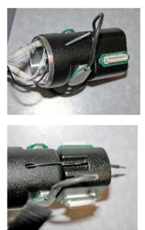
5. Leave enough slack in the section of fiber between the encoder and connector modules to match the loop of the other wires. A small lightweight tie can be loosely attached to hold the fiber adjacent to the wires.
