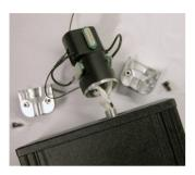
3. Carefully pull the FORJ away from the commutator face until the fiber is free.
