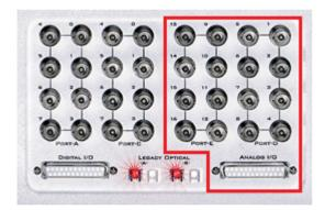
The RZ2 also includes onboard D/A for stimulus generation and experiment control, and A/D for input of signals from a variety of other analog sources.
