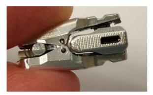
Firmly press and hold the **back** to open the headstage.
