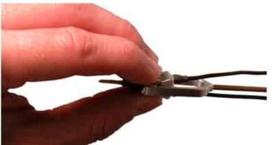
Position the headstage holder between the cables of the ZIF-Clip® headstage. The headstage should be completely secured in the holder.
