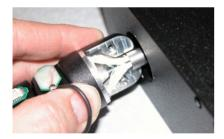
The plate should be just below body of the ACO32 and the encoder body should sit snuggly inside the lip of the clamping plates. Be careful not to pinch any wires or the fiber as the plates are tightened together.
