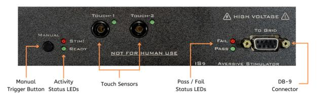
The iS9 generates small electrical currents for standard behavioral conditioning experiments, such as startle and Pavlovian fear response. Timing is precisely controlled for pairing the stim with other sensory cues or behavioral events. The iS9 is compatible with 3<sup>rd</sup> party behavioral boxes (Med Associates, Lafayette, and Harvard Apparatus).
