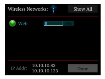
The Wireless Networks screen is displayed by touching WiFi on the System Setup screen. Available networks that have been used or previously configured are displayed in the main area of the screen. Selecting a network from the list displays network information and enables the user to connect to the network, forget the network, or cancel configuration of the network.
