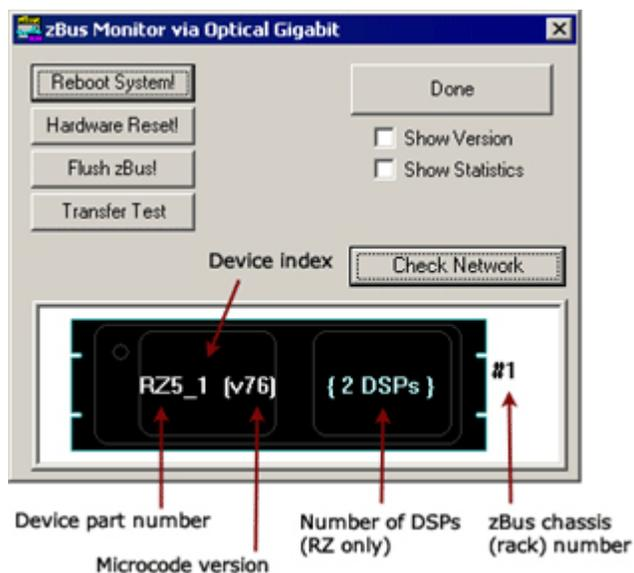
The device part number and index for each device along with the zBus chassis numbers are displayed in the system diagram. The version number of each programmable device's firmware (TDT Microcode) is also displayed within parentheses next to each device. See "Updating the Microcode" on page 22-6, for more information about the microcode.
