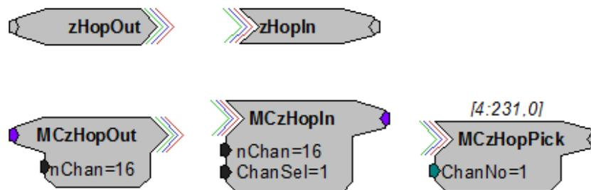
In RPvdsEx data is transferred across the zHop bus using paired zHop components, including zHopIn, zHopOut, MCzHopIn, MCzHopOut, and MCzHopPick. Up to 126 pairs can be used in a single RPvdsEx circuit.
