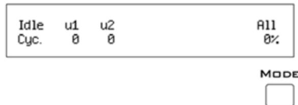
The front panel VFD screen reports detailed information about the status of the system. The display includes two lines. The top line reports the system mode, Run!, Idle, or Reset, and displays heading labels for the second line. The second line reports the user's choice of status indicators for each DSP followed by an aggregate value.
