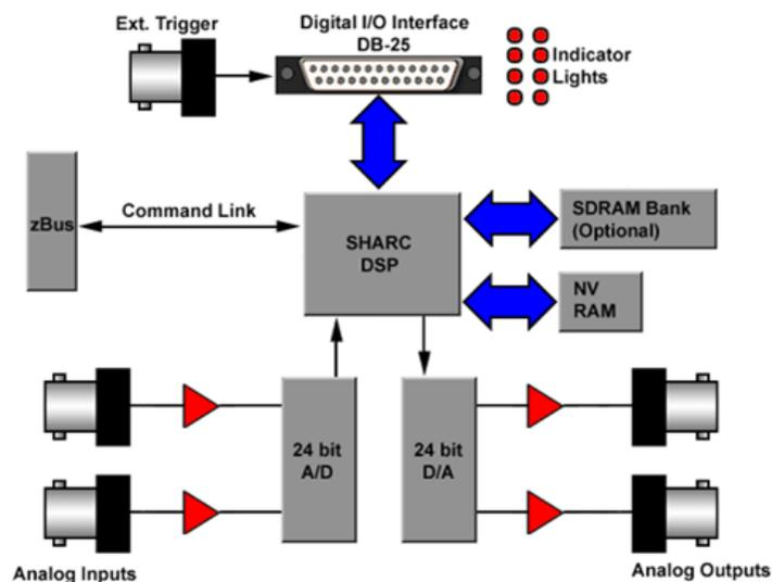
The RP2 is interfaced to the analog world via a two channel 24-bit analog to digital converter and a two channel 24-bit digital to analog converter. The RP2 system's I/O buffer handles +/- 10 Volt signals with excellent signal to noise performance. The RP2 contains a 100 kHz (50 kHz BW) A/D and a 200 kHz (100 kHz BW) D/
