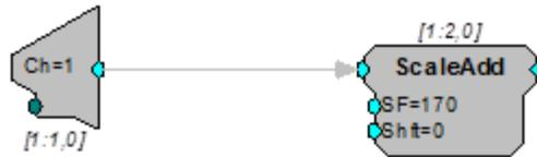
A parameter tag may be used to allow the scale factor of the channel input to be modified at run-time.
