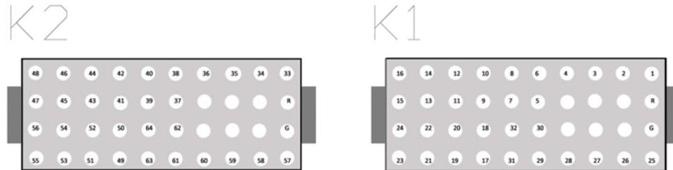
40-pin Samtec FOLC high density socket strips (pinouts looking into the connector)
