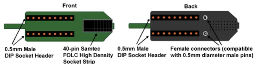
**Pinouts are looking into the connector and reflect the preamplifier channels.**
