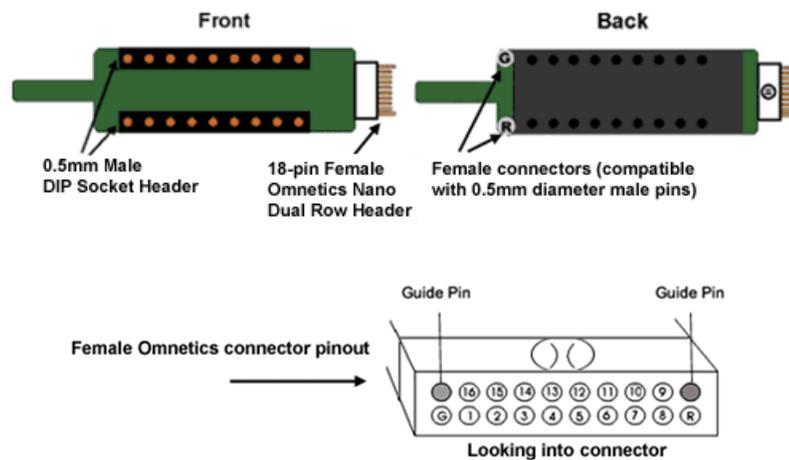
**Pinouts are looking into the connector and reflect the preamplifier channels.**
