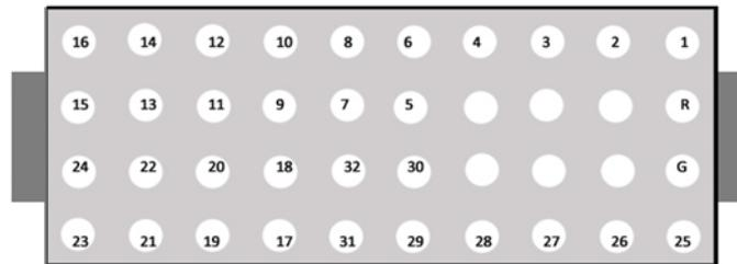
40-pin Samtec FOLC high density socket strip (pinout looking into the connector)
