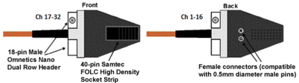
**Pinouts are looking into the connector and reflect the preamplifier channels.**
