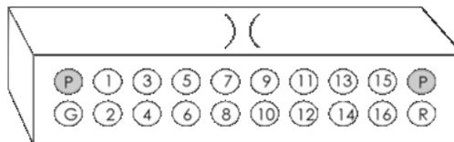
18-pin female Omnetics nano dual row header (pinout looking into the connector)
