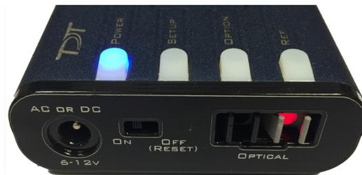
Use the provided fiber optic pair (black cable, white connectors) to connect the OPTICAL port on the preamplifier to the optical input port on the base station.
