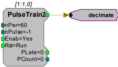
The PulseTrain2 component sends out a pulse every 60 samples. The output from the PulseTrain2 is sent to the Trigger line on a latch. Therefore the output from the latch is updated once every 60 samples. This generates an updated output that more closely matches the data transfer rate of the motion tracker. The output can then be sent to a head related transfer function (HRTF) coefficient generator (see “Using the HTI3 with HRTF Filters” on page 18-15).
