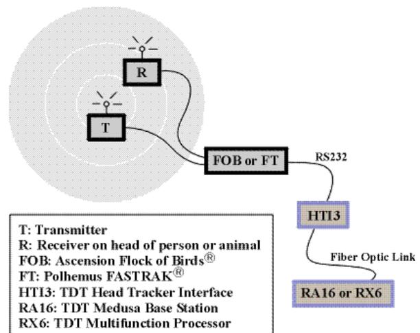
**Note:** The XYZ space is absolute distance from the transmitter while the AER information is relative to the boresight point.
