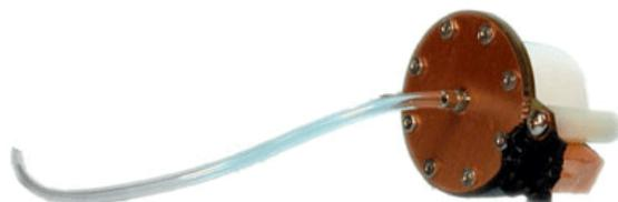
The EC1 includes a small piece of Tygon® tubing coupled to the output. The tubing will transfer the signal best when it is kept straight. Note that the speaker performance is dependent on the coupling system used and the ear of the animal. Users should test the device under experimental conditions to ensure it meets their requirements. Technical Specifications measured under specific controlled conditions are provided for comparison purposes.
