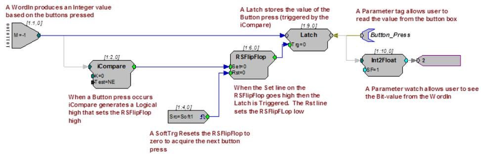
In the previous examples all button presses are acquired, that is, if a person presses buttons simultaneously there is the chance that both responses will be obtained. This will happen infrequently with circuits that use an iCompare and Latch, but it is still possible. In some cases the user will want to determine if the proper button press was acquired or wait until a particular button press has happened. Additional circuitry can be added that checks for this.
