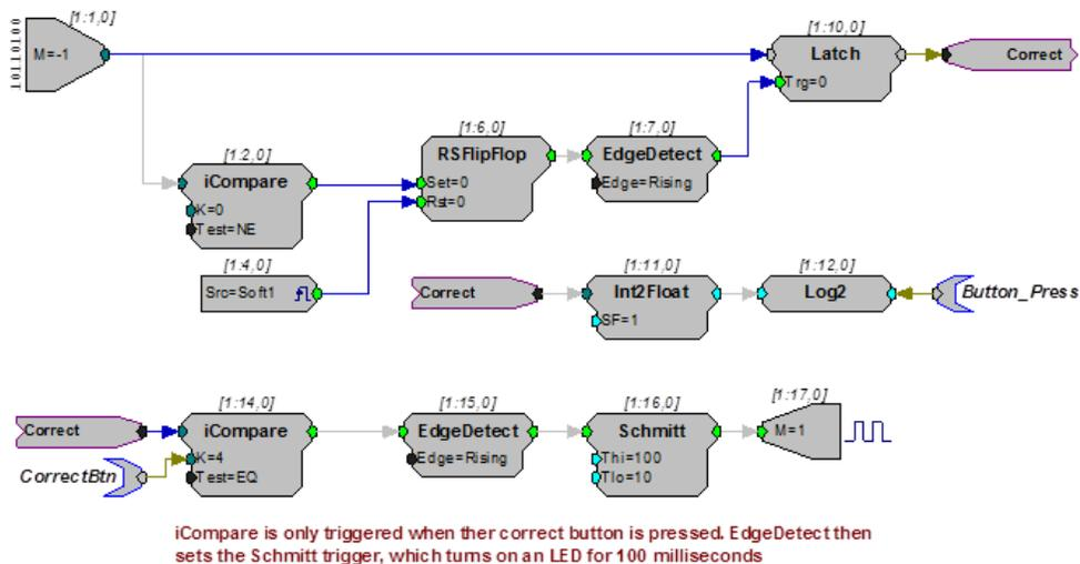
In this example, the top part of the circuit detects if a button is pressed. The button press value is also translated into a value representing which bit was read. For example, if the bit in bitmask value is 16, then Log2 converts the value to 4. This lets the user determine, via the Button\_Press parameter tag, that bit 4 was high.
