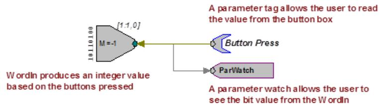
In this example, the user would continuously poll the component, from a program that acquired the value from the ButtonPress parameter, to determine which buttons are pressed. A simple circuit like this may be required if the RP2 that controls the button box is also used for stimulus presentation.
