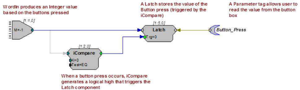
In this example, the WordIn produces an integer value based on the buttons pressed. When a button press occurs, an iCompare generates a logical high that triggers the Latch component. The Latch stores the value of the button press until the next button press occurs. The Button\_Press parameter tag allows the user to read the value from the button box. If only the first button press is important then a reset line should be included in the circuit to rest the Latch.
