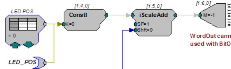
iScaleAdd adds the ON OFF DataTable value to the LED position value to turn the LED on or off
