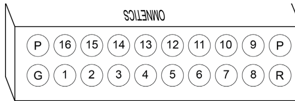
Side A pinouts are looking into the connector and reflect the preamplifier channels
