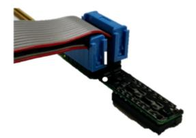
Align the silver marking on the headstage connector with the upper silver dot on the AC16LR. The red lines of the connector ribbon cable should be on the same side.
