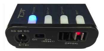
Use the POWER button on the top of the Medusa4Z to turn it on and off. There is an ON/OFF (RESET) switch on the side which completely disconnects the battery and loses all user settings. You should only use the ON/OFF (RESET) switch if storing the Medusa4Z for an extended period of time.
