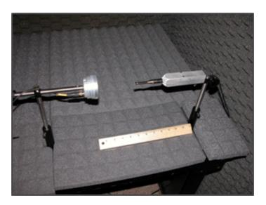
Figure 4 - A sound chamber used for testing and calibrating speakers
