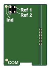
Connecting a jumper between the headstage reference pins and either the REF1 or REF2 pin connects the headstage reference to the desired probe reference (see table left for more information).
