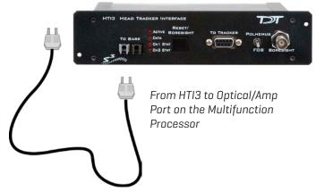
**Important!** Both ends of the cable are the same but the two sides of the connector are different. See the illustrations below to determine the correct way to make the connection for the Headtracker Interface.
