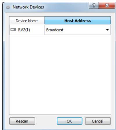
**PC Tools.** RVMap software is installed with TDT drivers. It provides a simple visual interface to define regions and targets for video tracking using video snapshots sent from the RV2 to the PC [or over the network]. Region and target information is collected and transferred to the RZ for storage.
