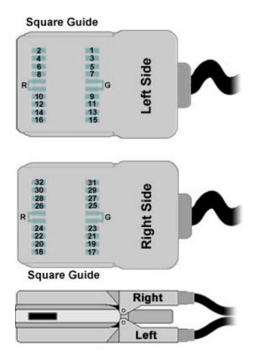
**Note:** A black square guide is used to align the headstage to ZIF-Clip® compatible connectors.
