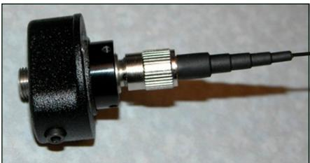
7. Slowly pull all of the excess fiber through the ACO32 until the FC/PC connector is inside the ACO32 and the fiber optic rotary joint plate can be attached to the ACO32 plate.
