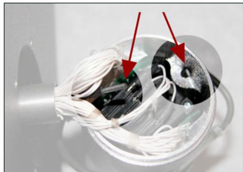
4. Pull the end of the fiber through the hole and insert it through the hole in the groove of the connector module.
