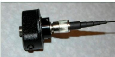
4. Disconnect the fiber from the joint.
