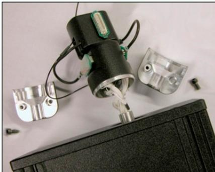
3. Carefully pull the FORJ away from the commutator face until the fiber is free.
