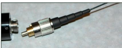
The fiber optic rotary joint (FORJ) assembly includes an FC/PC optical fiber connector and a single channel optical fiber threaded through the module. The FORJ assembly can be removed and re-installed by the user to allow for replacement of the optical fiber. The assembly supports use of fiber with a 1.25 mm cannula [tip].
