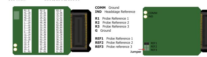
Pinouts are looking into the connector and reflect the preamplifier channels.
