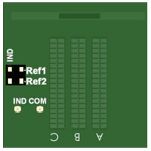
IND Headstage Reference Ref1 Probe Reference 1Ref2 Probe Reference 2 Com Ground
