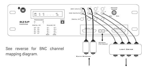
**Fiber Optic PZ Input Port.** The RZ5P is equipped with a fiber optic port for digitized input from a PZ amplifier or digital headstage manifold.
