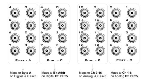
**Digital Input/Output.** Includes 24 bits of programmable digital I/O:
