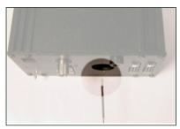
2. Slowly push the fiber through the hole until the end appears among the wires on the other side of the ACO32.
