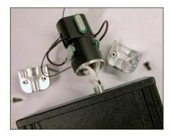
3. Carefully pull the FORJ away from the commutator face until the fiber is free.
