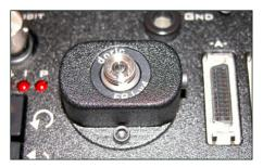
8. Attach the encoder clamping plates back onto the ACO32 shaft by tightening the screws. The plate should be just below body of the ACO32 and the encoder body should sit snuggly inside the lip of the clamping plates. Be careful not to pinch any wires or the fiber as the plates are tightened together.
