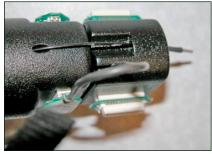
5. Leave enough slack in the section of fiber between the encoder and connector modules to match the loop of the other wires. A small lightweight tie can be loosely attached to hold the fiber adjacent to the wires.
