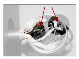
4. Pull the end of the fiber through the hole and insert it through the hole in the groove of the connector module.
